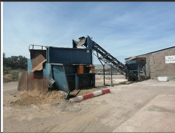
Crushing plant fitted with sprayers
